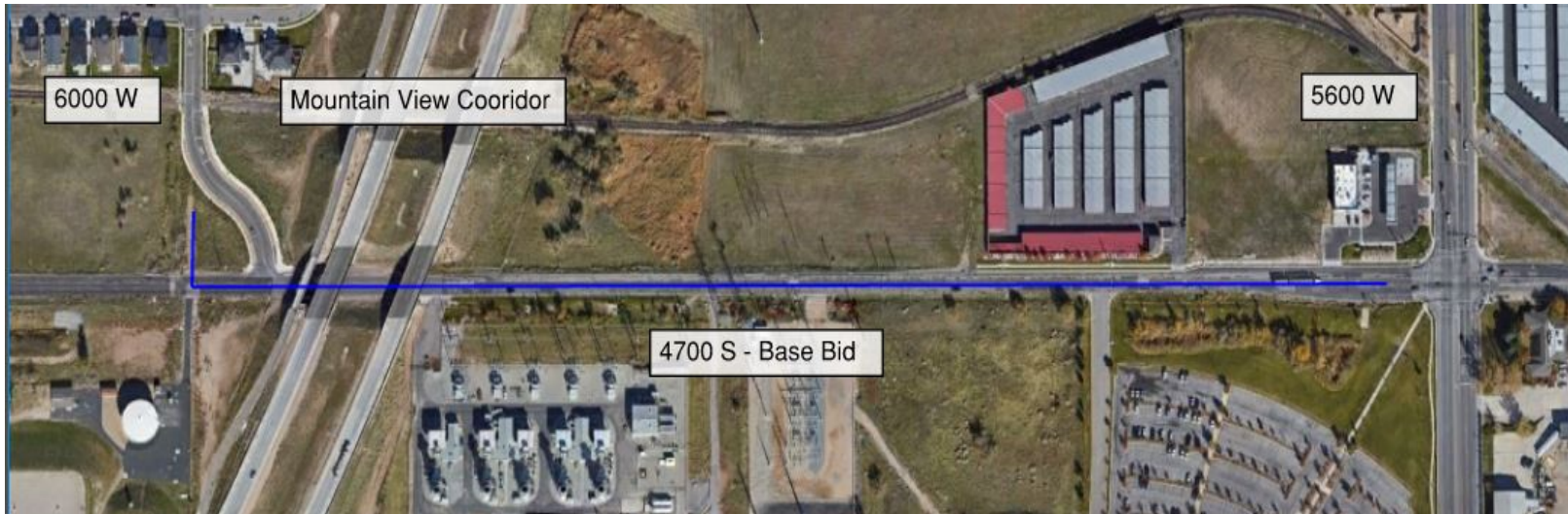
4700 South - Replacement of 3,250 feet of steel pipe from the 1970's.
