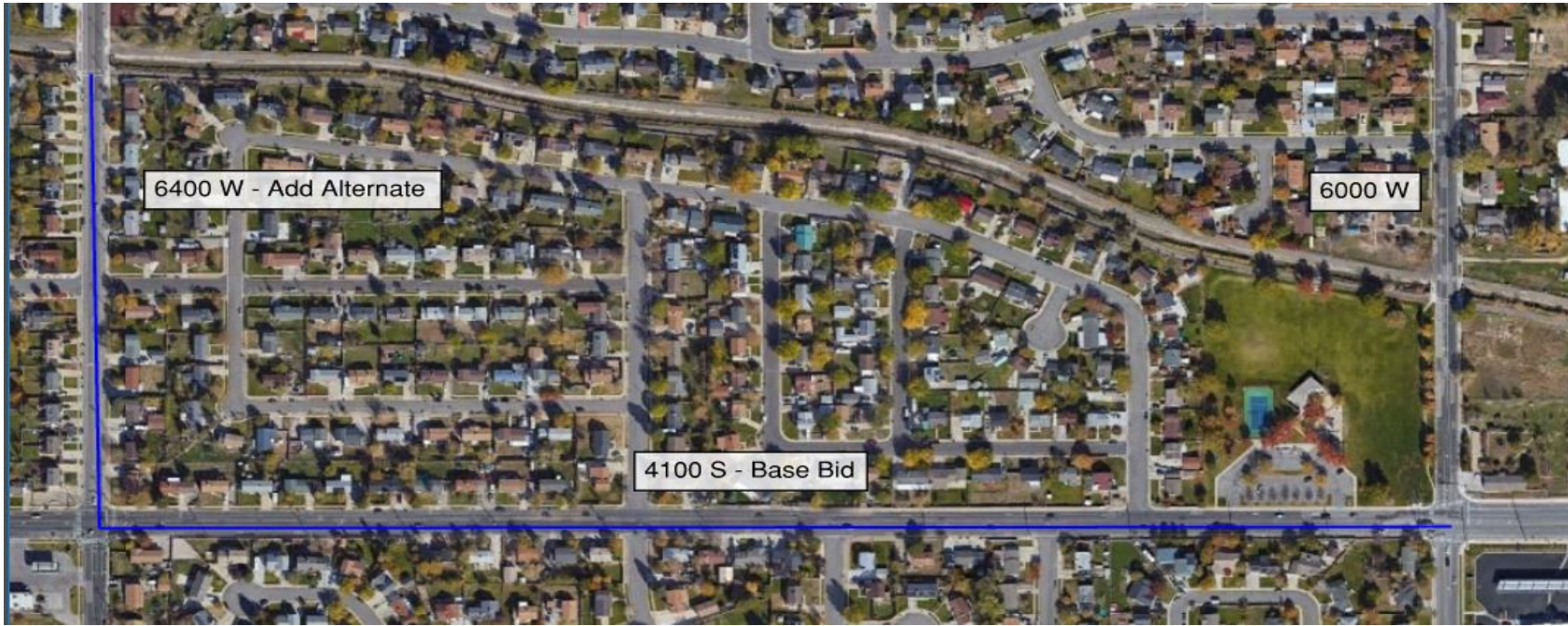
4100 South and 6400 West - Replacement of 4,175 feet of cast iron pipe from the 1950's.
