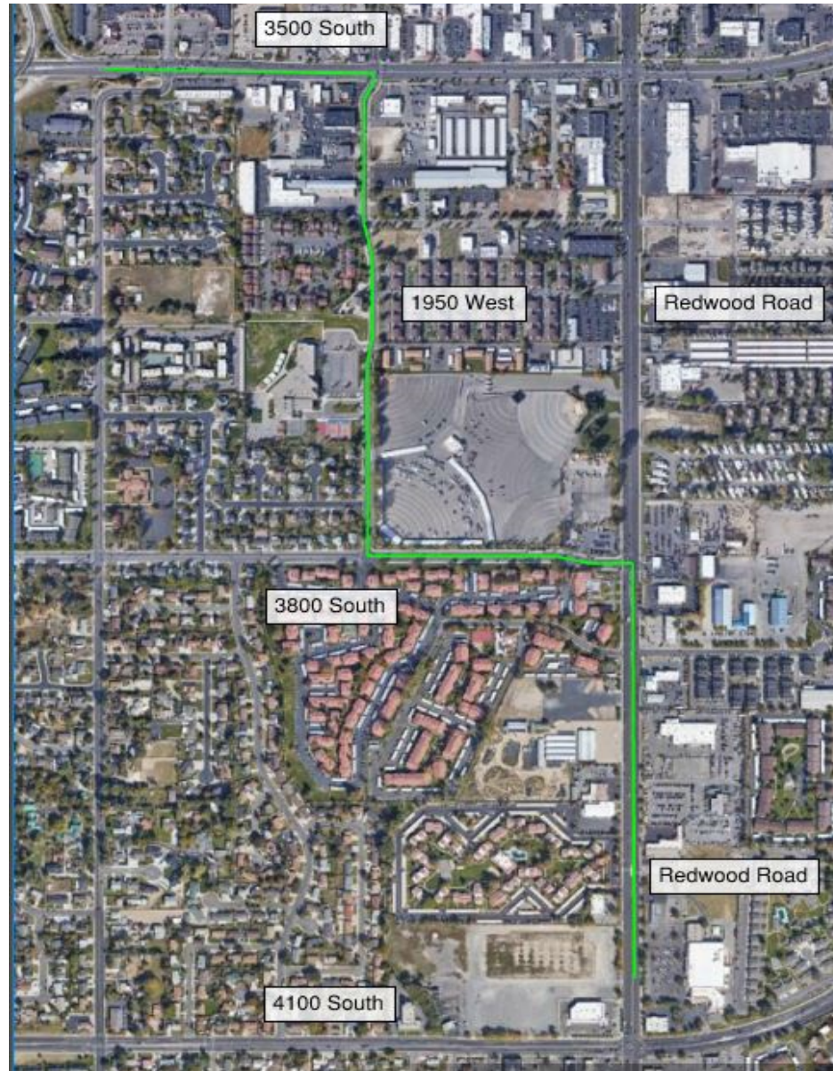
Redwood Road - Replacement of 7,950 feet of undersized pipe from the 1960's and 1970's.
