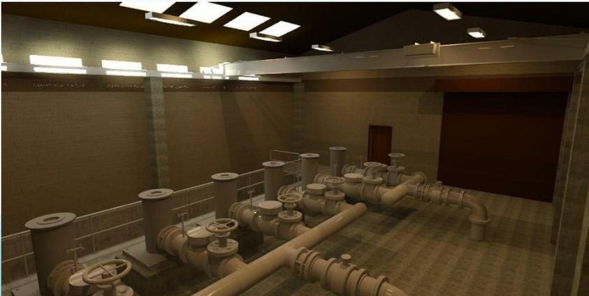
3-D BIM of interior of proposed Kent Pump Station Replacement.
