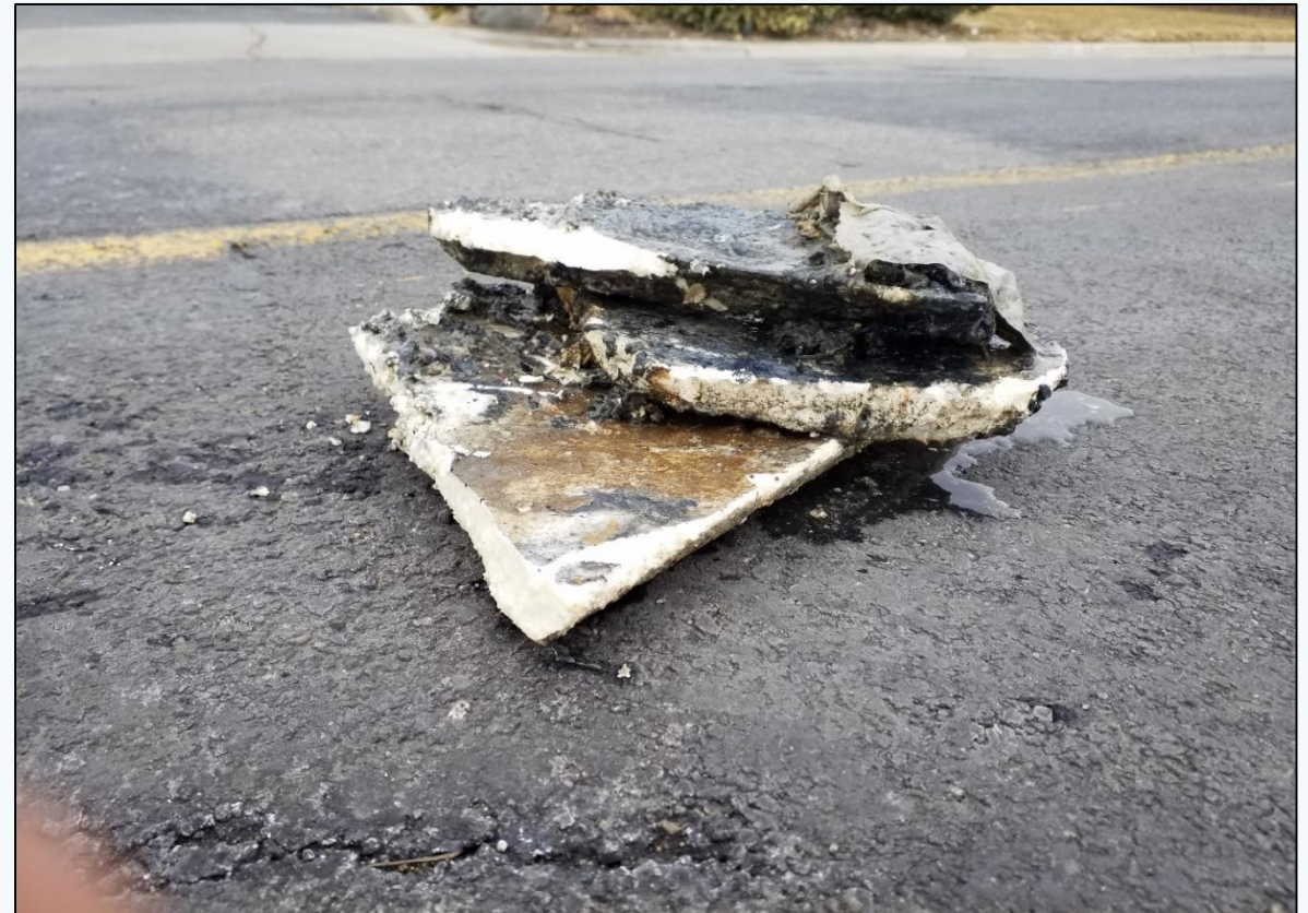
This image depicts some large, thick chunks of grease that were discovered and removed from a manhole, while performing our annual manhole inspections.
