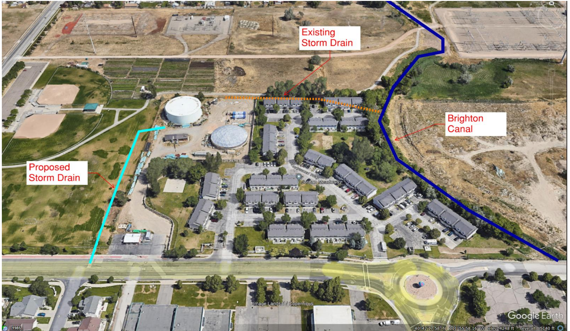
Fig 2: Aerial of Rushton Groundwater Treatment Plant Storm Drainage
