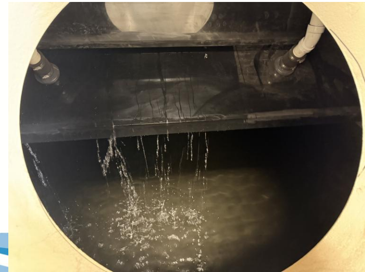
Anderson WTP Building bollard sleeves and pressure filter zone leak testing
